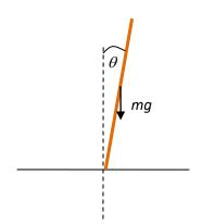
The torque provided by the weight about the point where the pencil touches the ground is  $mg\frac{L}{2}\sin\theta$ and so  $mg\frac{L}{2}\sin\theta = I\alpha$ . The moment of inertia is  $\frac{1}{3}mL^2$  and so  $\alpha = \frac{3g}{2L}\sin\theta$  or  $\frac{d^2\theta}{dt^2} = \frac{3g}{2L}\sin\theta$ .
